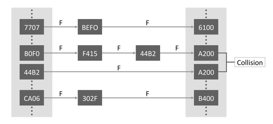
Only one hard disk access needed instead of one for each chain link
