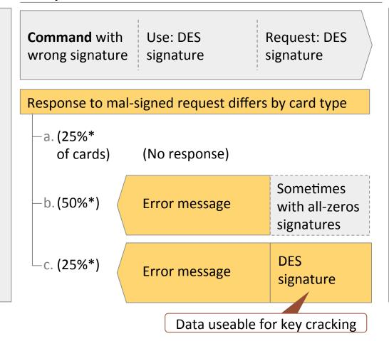
**SIM** card with DES key (prevalence of DES keys varies between operators; can be up to 100%)
