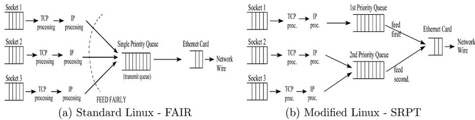
Fig. 5. Data flow in standard Linux (left) and in Linux with priority queuing (right).
