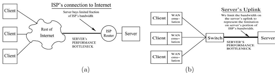
Fig. 2. (a) Server's bottleneck is the limited fraction of bandwidth that it has purchased from its ISP; (b) Our implementation setup models this bottleneck by limiting the server's uplink bandwidth.
